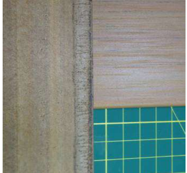
Figure 6 – Sample D rear face (left) held against the Tasmanian Oak colour sample. An eroded strip can be seen to the right of Sample D.
