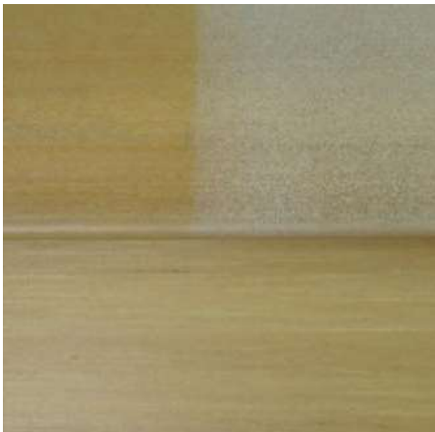
Figure 3 – Sample C front face (top) held against the Golden Oak colour sample. The exposed region of the front face of sample C can be seen top right.
