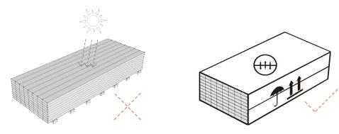
**THERMAL MOVEMENT :** INNOWOOD - Wood Composite products will expand and contract slightly with change in temperature. The amount of expansion and contraction varies according to the amount of change in temperature. The average expansion is expected to be controlled at 2mm per meter during a hot day if both ends are properly fixed with screws as per "INNOWOOD Installation manual.
